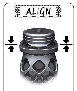
Just like with regular caps, our cap needs to be put on correctly in order to provide a leak-proof seal. Make sure it is not crooked or lopsided, and that it lines up with the bottle's neck ring, similarly to the image above.
